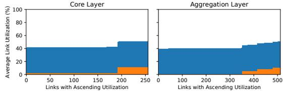
(b) Network link utilization when multicast messages are randomly routed to one of the eight ToR switch sequencers
