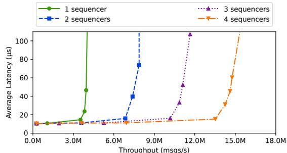
(b) Latency and throughput of Hydra with increasing number of end-host Hydra sequencers
